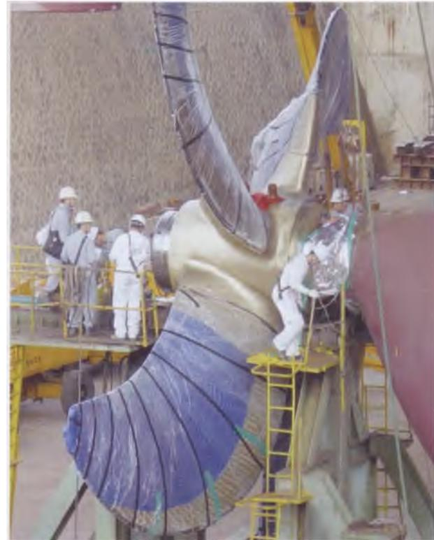
Inspectors are present during the installation of a propeller
